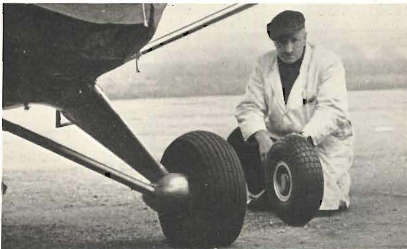
Oversize low-pressure tyres with large contact area enable the Workmaster to use muddy airstrips without fear of bogging down or nosing over. An engineer holds a wheel taken from a typical spray plane to show the extra size of the Workmaster's wheel.
