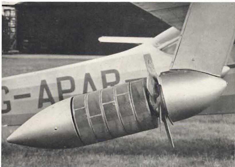
Shown above is the Micronair Rotary Atomiser, large numbers of which are in service in many countries. The Micronair offers a wide range of droplet sizes all of which can be accurately controlled.
