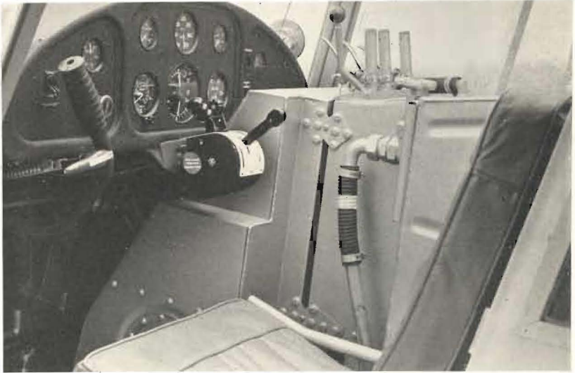
The 100 gallon tank is positioned alongside the pilot for safety. Adequate provision of large inspection panels makes cleaning easy. Built-in baffles add strength and eliminate surge during manoeuvres. Entire tank is removable through top canopy and is all welded using a technique to combat corrosion and fatigue cracks.
